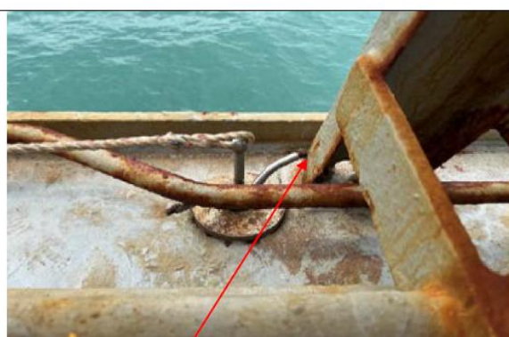
Unable to tighten the plug due to obstruction for turning lever
