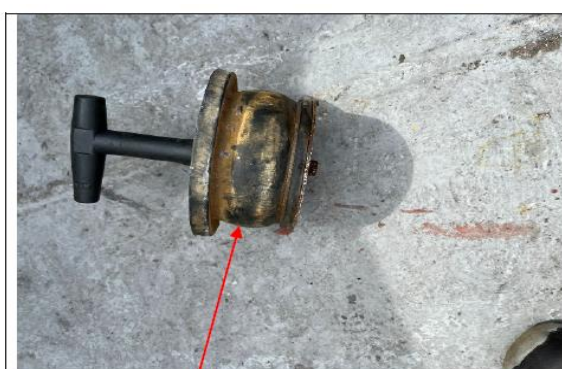
Diaphragm is not compressing/inflating on turning the tightening knob
